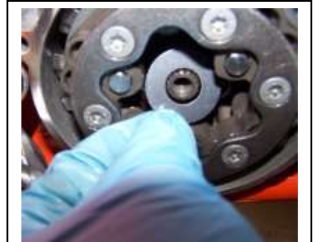
REMOVE OEM STOP DISK AND CLUTCH
